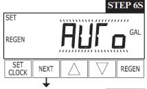
**Step 6S** – Set "AUTO" for estimating reserve volume capacity and total volume capacity automatically.
