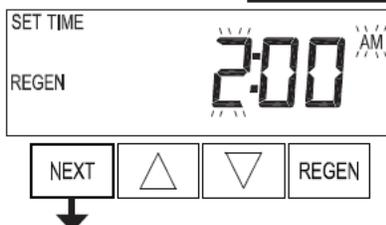
**Step 3I** – Next Regeneration Time (hour): Set the hour of day for regeneration using ▲ or ▼. The default time is 2:00. Press NEXT to go to step 4I. Press REGEN to return to previous step.
