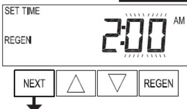
**Step 4I** – Next Regeneration Time (minutes): Set the minutes of day for regeneration using ▲ or ▼. Press NEXT to exit Installer Display Settings. Press REGEN to return to previous step.
