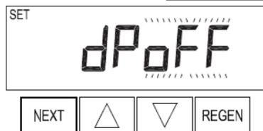
**Step 3CS** – Select “dP OFF” so that no outside signal is used to initiate a regeneration.
