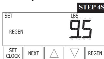
**Step 4S** – Enter the pounds of salt usage per regeneration. Press NEXT to proceed to Step 5S or Press REGEN to return to previous step.
