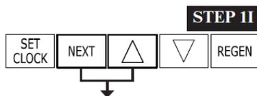
**Step 1I** - To enter Installer Display press NEXT and ▲ simultaneously for about 5 seconds and release.
