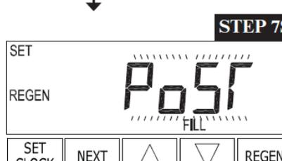
**Step 7S** – Set “PoST” Refill location using ▲ or ▼ to refill the brine tank immediately after the final rinse. Press NEXT to go to Step 8S. Press REGEN to return to previous step.
