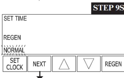
**Step 9S** – Set “NORMAL” for the regeneration time. Press NEXT to exit Softener System Setup or Press REGEN to return to previous step.
