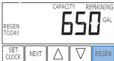
**Immediate Regeneration:** - Press and hold "REGEN" button for more than 3 seconds. Press "REGEN" button to advance the unit to next cycle in regeneration.
