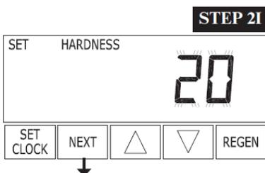
**Step 2I** – Hardness: Set the amount (gpg) of hardness using ▲ or ▼. Press NEXT to go to step 3I. Press REGEN to exit Installer Display Settings.
