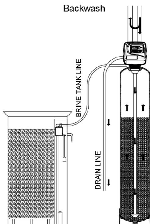
In **Backwash** Cycle water flows in upflow direction, the water enters the tank from bottom distributor and collected by upper basket. This operation lifts the bed and wash the resin. The water goes out through the drain line.
