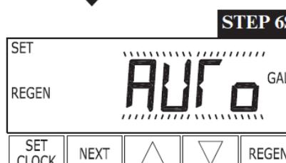
**Step 6S** – Set “AUTO” for estimating reserve volume capacity and total volume capacity automatically.
