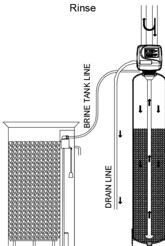
In **Rinse** Cycle water flows rapidly in downflow direction through the resin to the drain. This cycle washes the excess sodium from the resin particles.
