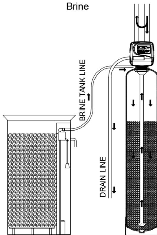
In **Brine** Cycle water flows in downflow direction which siphon the brine solution from brine tank and slow rinse water goes to the drain.
