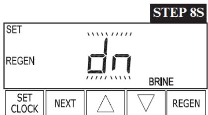
**Step 8S** – Select “dn” for downflow brine cycle using ▲ or ▼. Press NEXT to go to Step 9S. Press REGEN to return to previous step.
