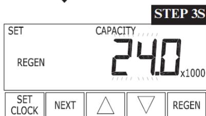
**Step 3S** – Enter the softening grains capacity given in specification sheet according to the salt usage.
