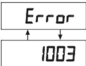
This error screen and error number will toggle. Contact Service Technician or Excalibur to report the error code.
