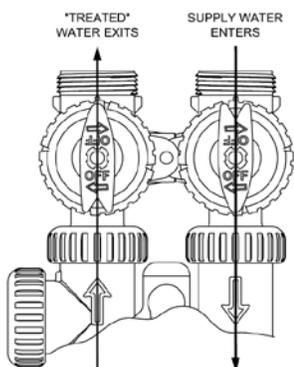
The bypass valve handle must be in the direction of flow and engraved arrows on control valve.
