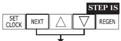
**Step 1S** - Press NEXT and ▼ simultaneously for 5 seconds and release.
