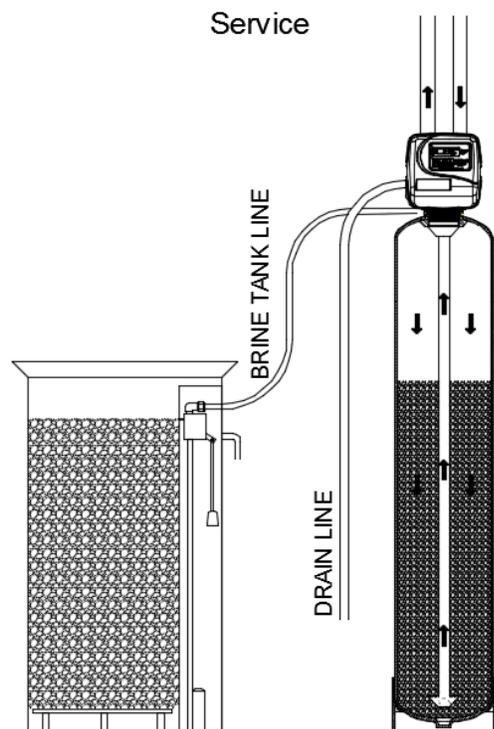
In **Service** Cycle water flows through the upper basket and flows down to the bottom distributor. In this operation hardness of water is removed by resin.
