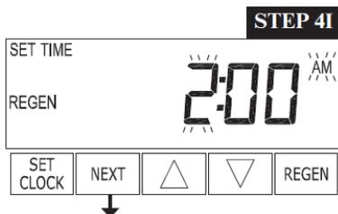
**Step 4I** – Next scheduled regeneration time (hour): Set the hour of day for regeneration using ▲ or ▼. (Usually 2:00AM or when the predictable flow is minimum) Press NEXT to go to step 5I. Press REGEN to return to previous step.
