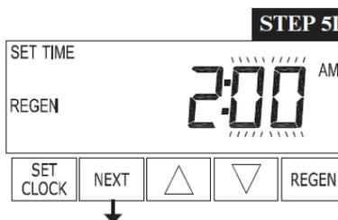
**Step 5I** – Next scheduled regeneration time (minutes): Set the minutes of day for regeneration using ▲ or ▼. Press NEXT to exit Installer Display Settings. Press REGEN to return to previous step.
