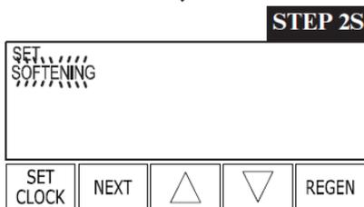
**Step 2S** – Choose SOFTENING using ▲ or ▼. Press NEXT to go to Step 3S. Press REGEN to exit OEM Softener System Setup.
