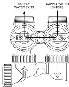
The bypass valve handles must be turned towards the center as shown above
