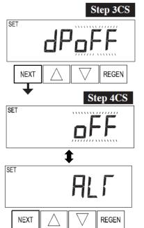
**Step 3CS** – Select "dP OFF" so that no outside signal is used to initiate a regeneration.
